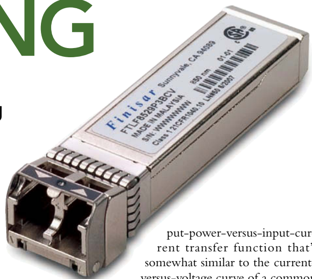
Optical transceivers require measurements and tuning for optimal output power. Courtesy of Finisar.
