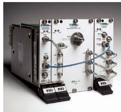
Instruments such as this 14-GHz vector signal analyzer have proven the viability of PXI for high-end RF communications test applications.
