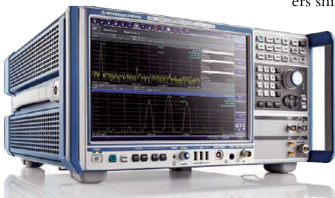
A spectrum analyzer can reveal the frequencies of offending emissions. Courtesy of Rhode & Schwarz.
